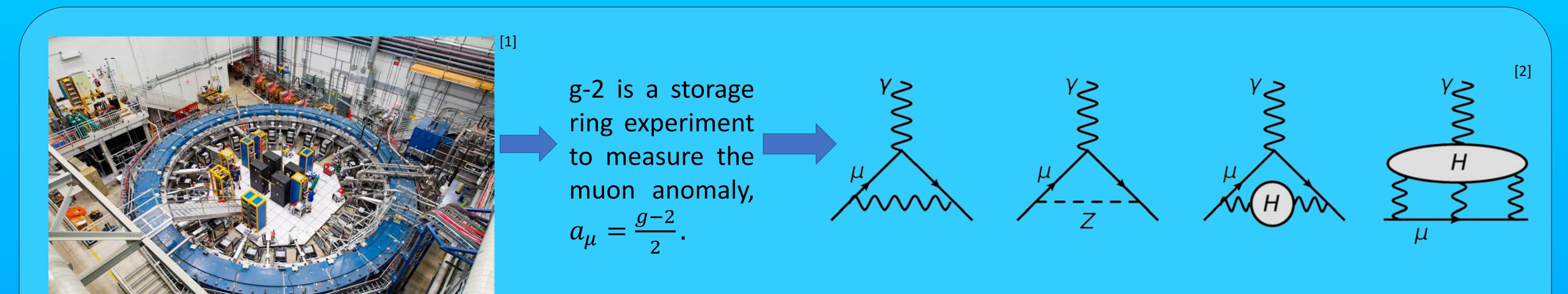
g-2 investigates the behaviour of the muons in a B-field. The g-factor relates the magnetic dipole moment (MDM) of a particle to its spin.  $\eta$  is analogous to the g-factor – it relates the electric dipole moment (EDM) of a particle to its spin.
