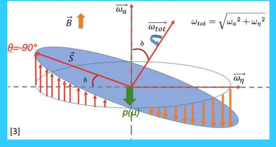
If present, a muon EDM causes the precession plane to tilt towards the centre of the storage ring.
