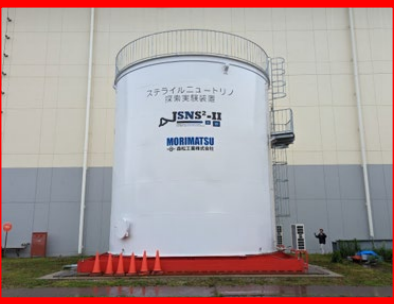
(JSNS 2 -II: New detector) 32t GdLS fiducial (6.2m dia. x 6.2m (h) ~230 10" PMTs)
