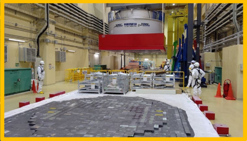
(JSNS 2 ) 17t GdLS fiducial (target) detector (4.6m dia. x 4.0m height, 120 10" PMTs)
