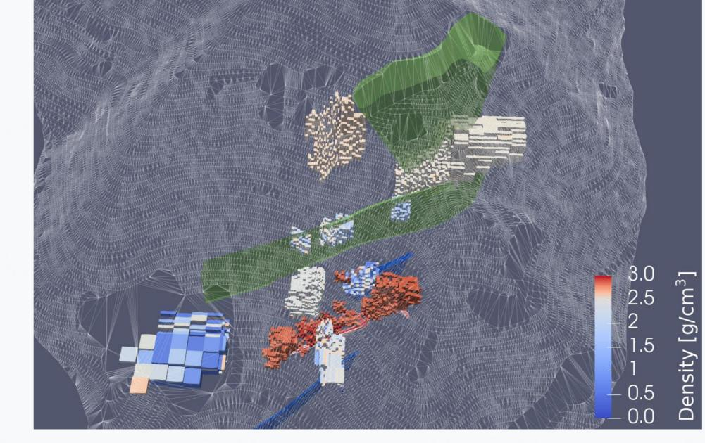
Survey results at a gold deposit using the new algorithm. Green and blue surfaces: ore body models. The surface in B5: the model of a slate. • Discovered four mined-out areas; half of them are confirmed by the documentation. Reconstructed the slate whose density are slightly different from the bulk density.
