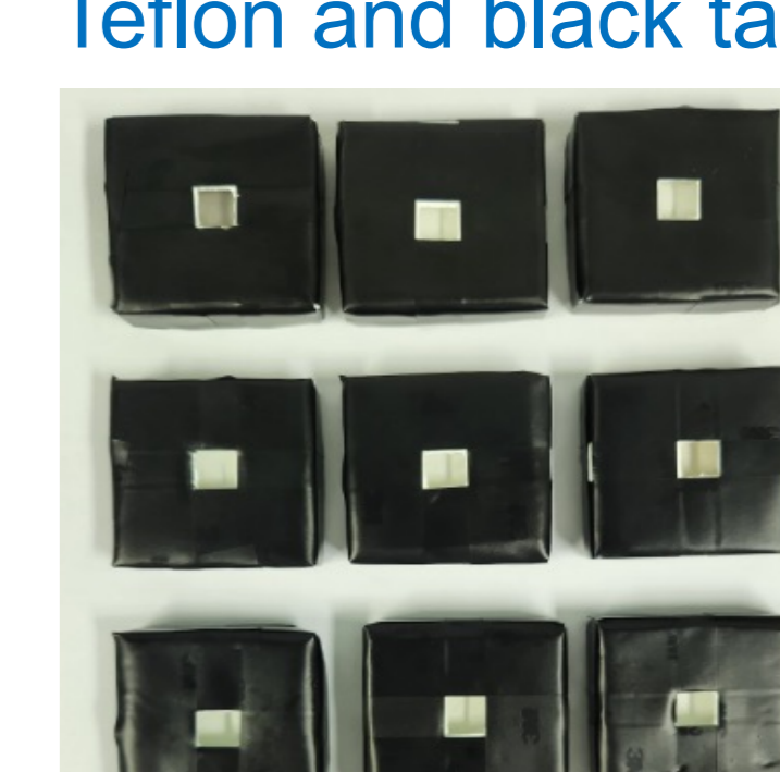
Glass tiles wrapped with Teflon and black tapes
