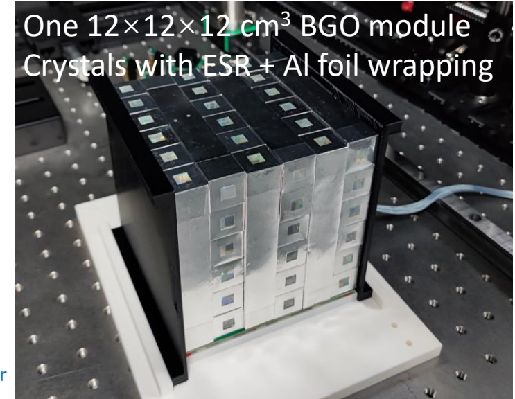
Support structure design and module assembly test
