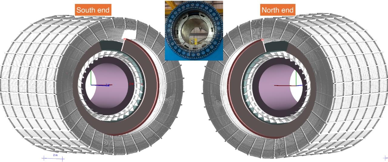
Precision simulation is crucial for determining the material budget and the energy sampling fraction.
