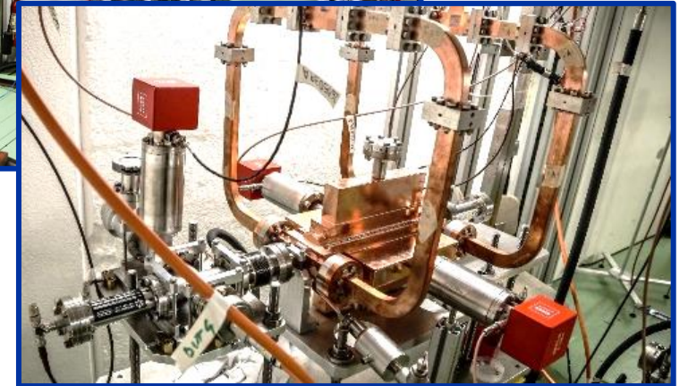
Figure: Exterior of the X-band high gradient test facility (top) and an X-band structure being tested (bottom).
